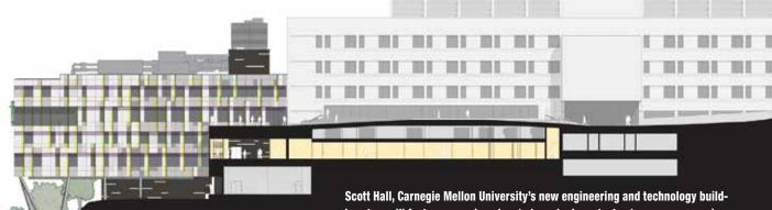
Scott Hall, Carnegie Mellon University's new engineering and technology building, *top*, will feature one wing elevated on sloping, steel columns over a ravine, while the other wing will fill in a sunken service courtyard. The new structures, *above*, will be surrounded by other science and engineering buildings.
