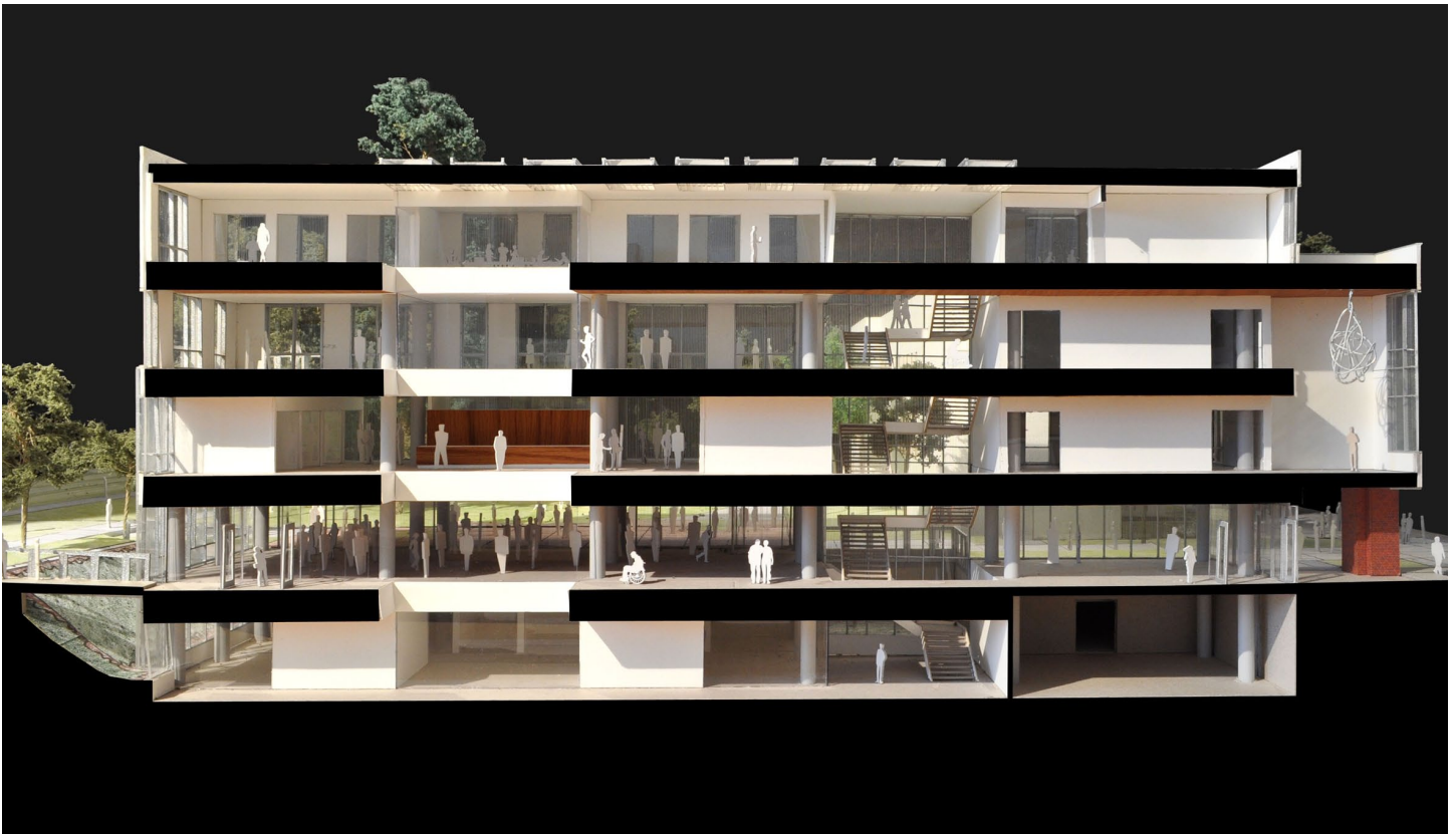
Scale model in the studio: a sectional study of natural daylight, circulation and open spaces (UO Tykeson Hall) by OFFICE 52.
