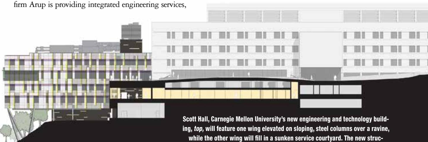
**Scott Hall, Carnegie Mellon University's new engineering and technology building, top, will feature one wing elevated on sloping, steel columns over a ravine, while the other wing will fill in a sunken service courtyard. The new structures, above, will be surrounded by other science and engineering buildings.**
